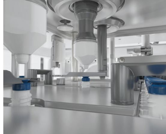
Integrated aseptic zone ensures the spout and plug are kept sterile throughout the filling process.
