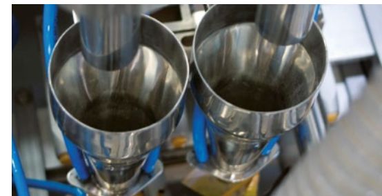
Wide sachet opening, enabling higher filling grade.
