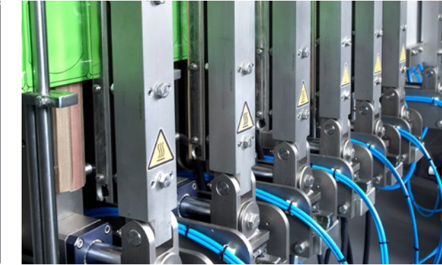
Parallel motion of the vertical sealing bars enables improved sealing quality and easier maintenance.
