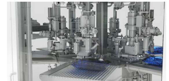
Rotary filling increases fill speeds up to four times over traditional linear filling.
