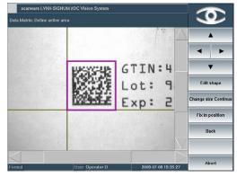
Quiet zones around the code are necessary for correct reading. For ideal reading, the software automatically includes these and provides a visual representation.
