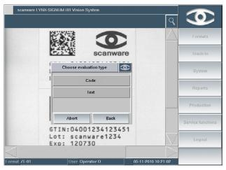
The teach-in can be configurated and consequently is very fast. Firstly, the print type to be inspected is chosen. Thereafter, only the parameters relevant to the type of print need to be taught.
