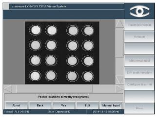
During teach-in, the system automatically generates evaluation parameters. These are calculated based on images and error images and can be adjusted by the user if desired.
