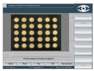
Automation of the teach-in simplifies the process so production can start in minimum time. Object position, blister geometry and product color are recognized automatically. A manual teach-in is also possible.
