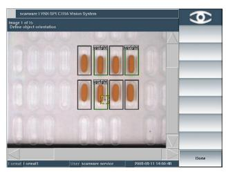
The recognition of upright objects reduces product ejections. Upright objects are identified as correct rather than ejected as too small.
