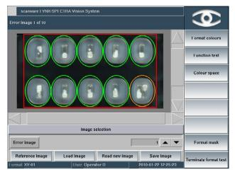
Using x/y measurement is useful for various products, for example Medical Strips. For hard gel capsules with heterogeneous filling, varieties in distribution of products within the capsules can be evaluated.
